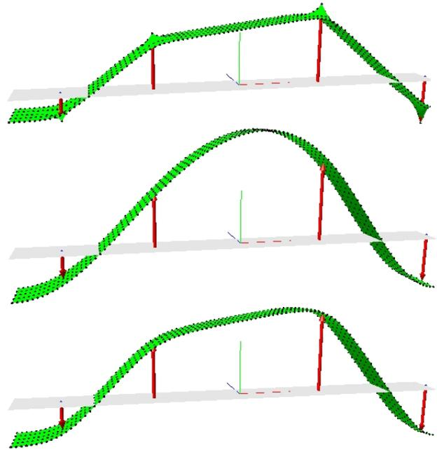
Figure 8: Interpolation of displacement constraints. Laplacian( $\gamma_1 = 1$ ,top), bi-Laplacian ( $\gamma_2 = 1$ ,middle) and mixed ( $\gamma_1 = 1, \gamma_2 = 0.1$ ,bottom)
