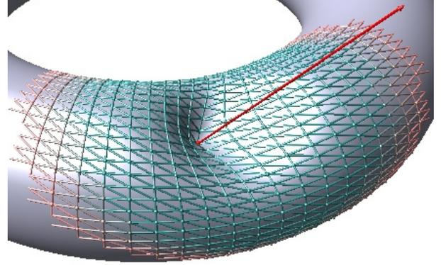
Figure 3: Automatically self-adjusting domain. Blue is the domain and red is a transition domain needed in the intermediate computation stage. All other vertices are not used.
