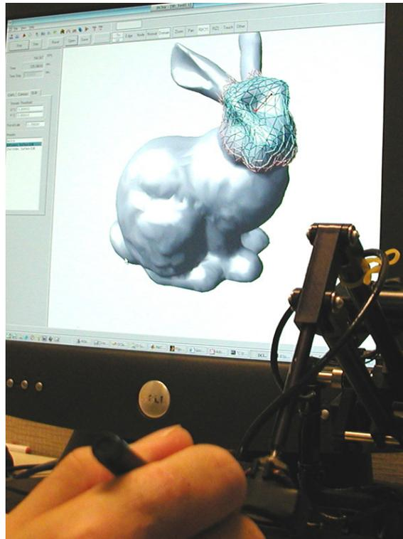
Figure 1: A user poking bunny with PHANToM. The PDE is solved in realtime by using self-adjusting active domain around the contact point.
