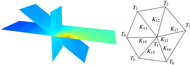
Figure 2: Heat diffusion over a non-manifold triangle mesh(left). An illustration of the  $\mathbf{K}\{T\}$  operation(right).
